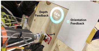
**Figure 5:** Users are given perpendicularity (right) and depth (left) feedback while drilling. The drill's rangefinder array ensures that the UI maintains a constant size and aspect ratio.
