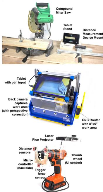
**Figure 3:** Augmented miter saw (top), augmented CNC router (middle), augmented drill (bottom).
