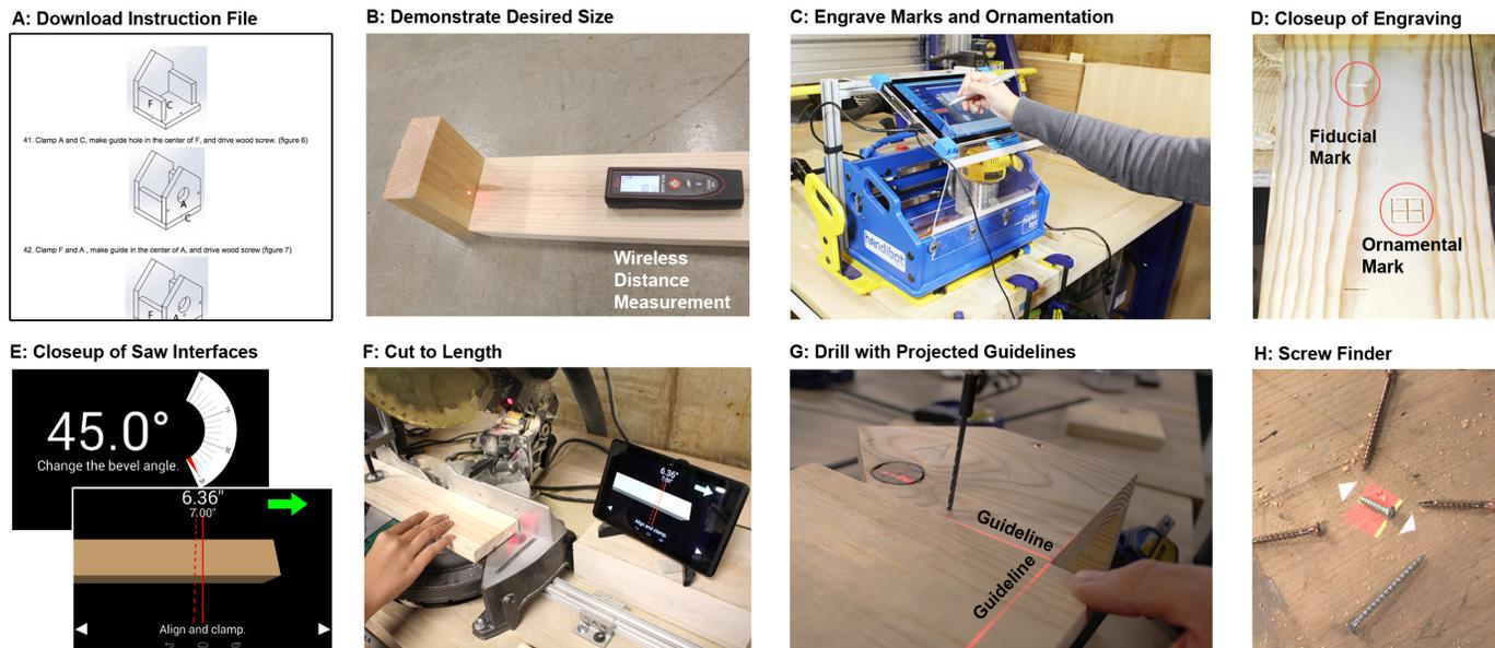
**Figure 2:** To complete a Drill Sergeant project, a user finds a model (a) and sizes it, measuring their desired final location (b). For this birdhouse, the user engraves a decorative pattern and fiducials (c, d), cuts boards to length (e, f), locates drill positions (g), and identifies the correct fasteners (h).
